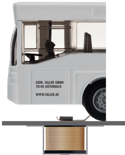
Fig. 11: South upwards: In analog Car System operation wrong polarity. In Car System Digital operation shift to slow speed.
