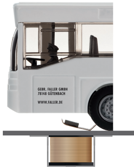
Fig. 12: North upwards: Correct polarity.
